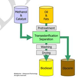
Since some methanol is still present in both the fuel and the glycerin layers at the end of the transesterification reaction, a process called **methanol recovery** may be conducted on both layers separately to recover the chemical. This methanol may be re-used in the next batch of fuel.
