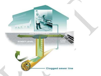
Redirecting used cooking oil collected from the public into biodiesel production reduces the amount of grease improperly poured down sinks and drains and reduces the number of sanitary sewer overflows.
